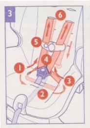
Thread the harness down through slot on left side of shell (1), across bottom of seat (2) and up through slot on right side (3). Make sure harness adjustment strap is between shell and harness strap.
