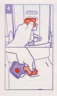
Insert buckle's metal clip up through the shell and pad. From the front, pull buckle free from shell and pad. Lock buckle plates into buckle for future use.
