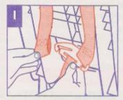
From the back of the seat, unfasten harness from splitter plate.
