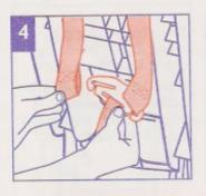
From the back of the seat, fasten harness to splitter plate.
