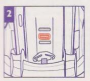
From under seat, pull metal clip down through slot in bottom of seat.
